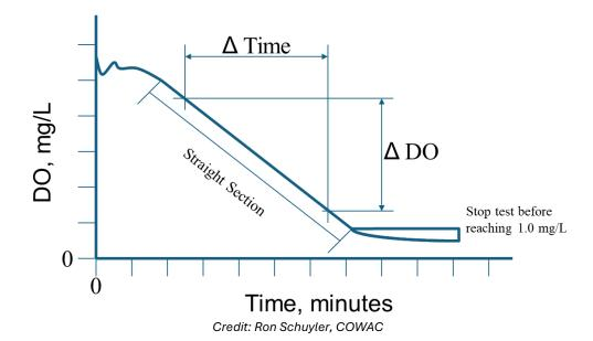
The oxygen uptake rate can be calculated from this chart – find two points along the straight section of the curve and divide the change in the DO by the change in time. This calculation shows how many milligrams of oxygen were consumed each minute. To obtain the SOUR results, more data is required – specifically the mixed liquor volatile suspended solids concentration (MLVSS).
