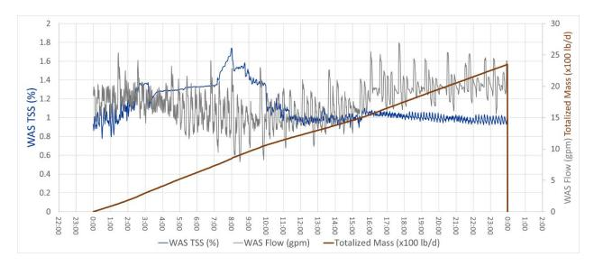
If the MLSS concentration is stable at your facility, a system like this allows operators to be engaged in the SRT/MCRT calculation but have accurate and precise wasting data. The program can be expanded to stop wasting once the total pounds have been achieved for the day or adjusting the WAS pump speed, so the total pounds are wasted over 8, 12, or 24 hours, ensuring that the proper amount of solids are removed from the system.
